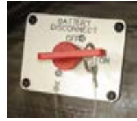
Battery Disconnect Switches
