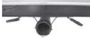
Black/Grey Tank Drain & Valves
